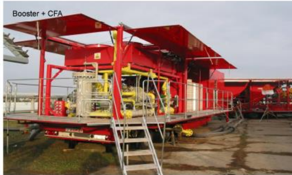
Figure 6.12 Compressors used by Eustream + booster unit
